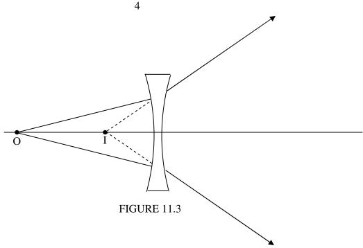
Figure II.3 shows a lens forming a virtual image of a real object. As before, light diverges from the real object, but no light converges to a real image. After refraction through the lens, the light is diverging from a point where the photons have never visited. The light is diverging from a virtual image.
