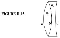
I have indicated the indices and the radii of curvature. The power (reciprocal of the focal length) of the first lens by itself is
