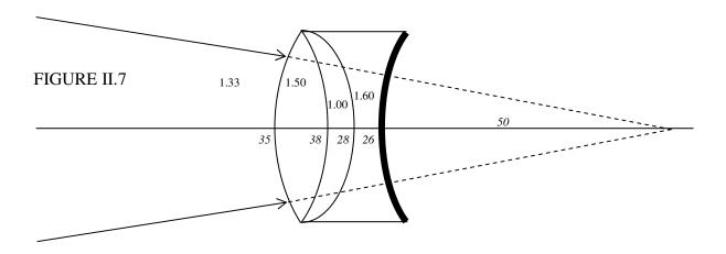
I have marked in the several refractive indices, and, in italics, the radii of curvature and the distance of the virtual object, in cm. Remember that, notwithstanding the drawing, we are assuming that all lenses are *thin* – that is to say that their thicknesses are negligible compared with other distances.
