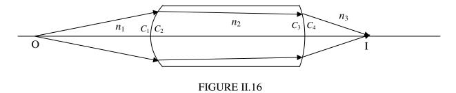
Figure II.16 shows a thick lens of index  $n_2$ , an object O and an image I. For good measure I have put a medium of index  $n_1$  to the left of the lens and a medium of index  $n_3$  to the right of the lens. If you are given the position of O, can you calculate the position of the image?
