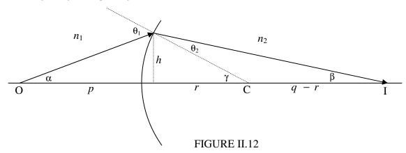
Figure II.12 shows a refracting interface of radius of curvature r separating media of indices  $n_1$  and  $n_2$ . I show a real object at O, a real image at I and the centre of curvature at C. Remember that angles are small and the "lens" is thin. We see that  $h = \alpha p = \beta q = \gamma r$ . By Euclid,  $\theta_1 = \alpha + \gamma$  and  $\theta_2 = \gamma - \beta$ , and by Snell,  $n_1 \theta_1 = n_2 \theta_2$ . From these, we obtain
