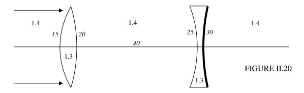
The two lenses are made of a very light solid whose refractive index is only 1.3. (I'm not sure if there *is* such a stuff!) and they are immersed in a liquid of index 1.4. That means that the convex lens is diverging. The second surface of the second lens is a reflecting mirror. I have indicated the radii of curvature, and the lenses are 40 cm apart. Parallel light comes from the left. Where does it come to a focus?
