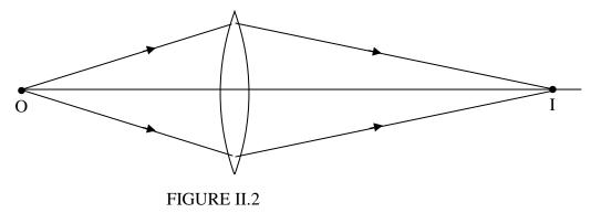
Figure II.2 shows a lens forming a real image of a real object, and I think it requires little explanation. Light diverges from a real object and it converges to a real image. Real photons of light depart from a real object, and real photons of light arrive at a real image.
