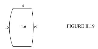
The lens shown is 4 cm thick and the refractive index is 1.6. The radius of curvature of the first face is 15 cm. An object is 32 cm to the left of the 15 cm face. Its image is real, inverted and magnified by 22. Determine the radius of curvature of the second face.
