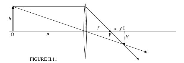
I have drawn two rays emanating from the tip of the object. One is parallel to the axis; after refraction it passes through the focus. The other goes through the centre ("pole") of the lens; since the lens is "thin", this ray is neither deviated not displaced. The two rays cross at the tip of the image. From two obvious pair of similar triangles, we see that
