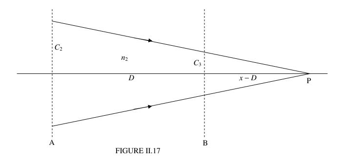
Figure II.17 shows a beam of light, in a medium of index  $n_2$ , converging to the point P, which is at a distance x from the plane A. The convergence of the beam as it leaves the
