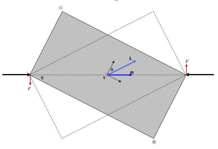
The torque on the plate can be represented as a *couple* of forces exerted by the bearings on the plate, each of magnitude  $\frac{\tau_3}{2\sqrt{a^2+b^2}}$ , or  $\frac{m(a^2-b^2)ab}{6(a^2+b^2)^{3/2}}\omega^2$ . Forces exerted by the plate on the bearings are, of course, in the opposite direction.
