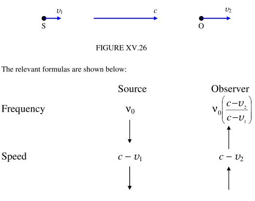
Wavelength  $(c - v_1)/v_0 \longrightarrow (c - v_1)/v_0$
