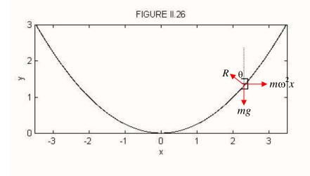
Suppose the liquid is circulating at angular speed  $\omega$ . A tea leaf floating on the surface is in equilibrium (in the rotating reference frame) under three forces: its weight *mg*, the centrifugal force  $m\omega^2 x$  and the normal reaction *R*. The normal to the surface makes an angle  $\theta$  with the vertical (and the tangent makes an angle  $\theta$  with the horizontal) given by
