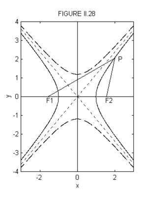
For example, in a Young's double-slit interference experiment, the *m*th bright fringe is located at a point on the screen such that the path difference for the rays from the two slits is *m* wavelengths. As the screen is moved forward or backwards, this relation continues to hold for the *m*th bright fringe, whose locus between the slits and the screen is therefore a hyperbola. The "Decca" system of radar navigation, first used at the D-Day landings in the Second World War and decommissioned
